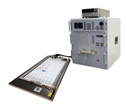
The test equipment for the reduction factor complies with the standards while allowing for a variable distance between the loop conductor and the cable under test.
