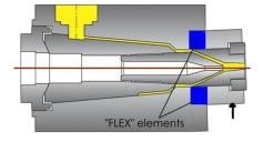
Cross head with the Microflex Flex element fully tight, correction is applied to the die.
