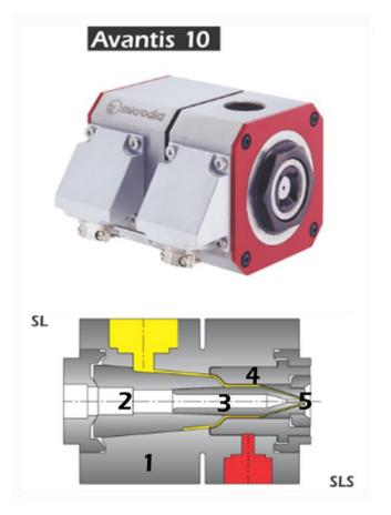
Due to the dimensional tolerance of each of the 5 parts assembled together, a slight deviation between tip [3] center and die [5] center is inevitable.
