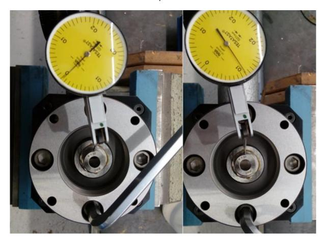
Bottom screw tighten. The die went down by 0.11 mm
